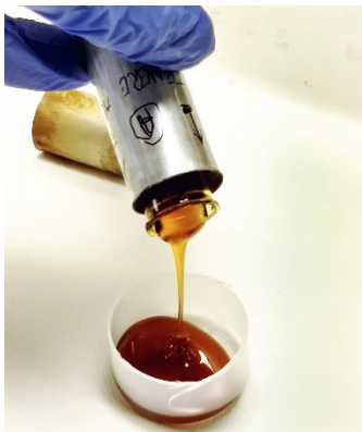
Lubricating oil irradiated at 8 MGy of dose in reactor. [M. Ferrari et al., NIM B vol.497 pp. 1-9 (2021)]
