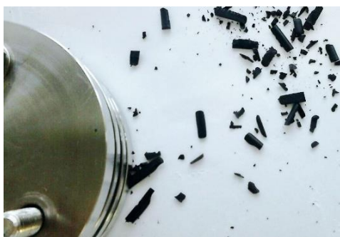
Structural failure of an elastomeric materials after irradiation in reactor at 3 MGy of dose.
